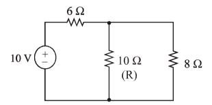
5. (a) In the following circuit, what should be the value of load resistance  $R_L$ , so that it can draw maximum power :  $\begin{tabular}{c} 5 \end{tabular}$
